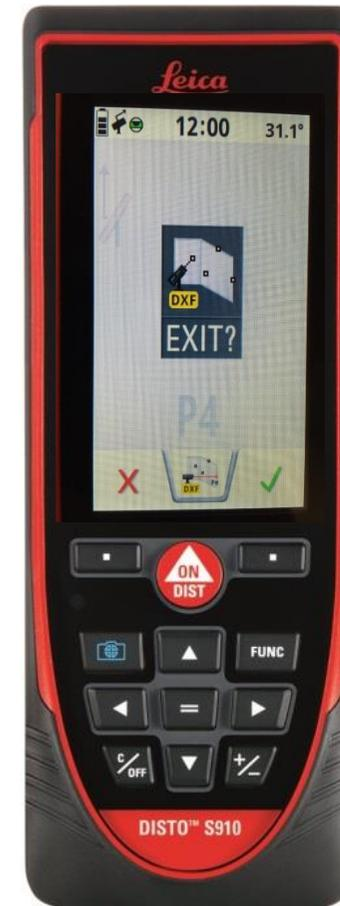
Either press the green check mark to accept recorded measurements and exit or press „X“ to keep measuring
