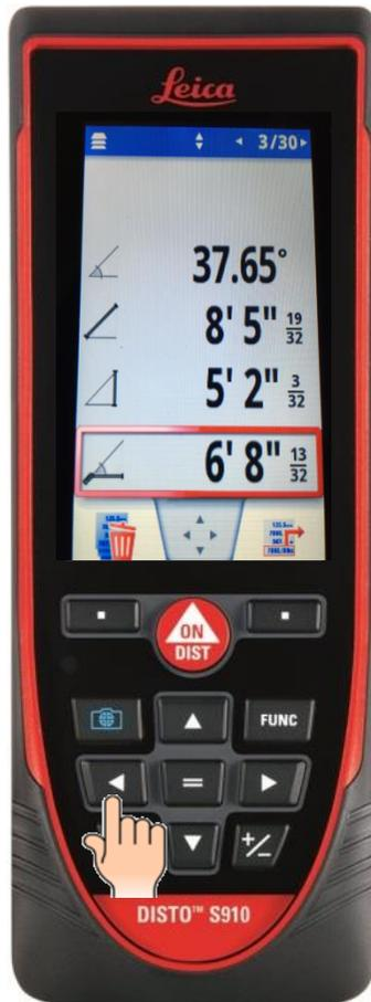
Go to measurement memory by pressing arrow key left or right
