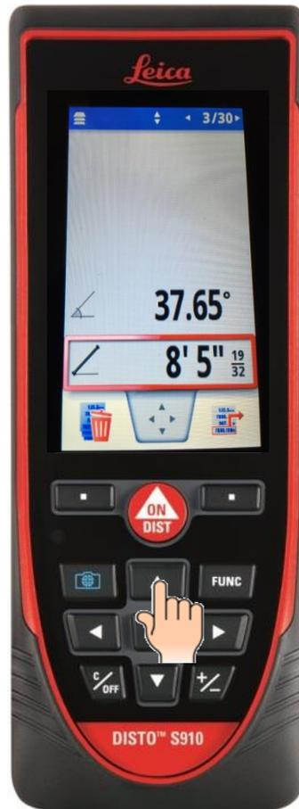
Scroll up to the measurement 8"5" 19/32 by pressing the up arrow key
