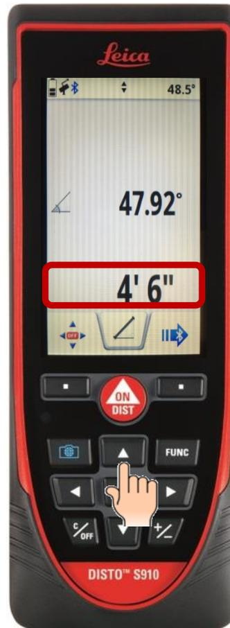
Press the up arrow keys to the disired measurement display.
