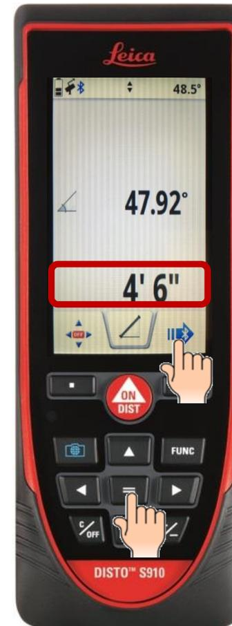
Press the touchscreen Bluetooth icon on the or press the equals key to transfer the measurement.
