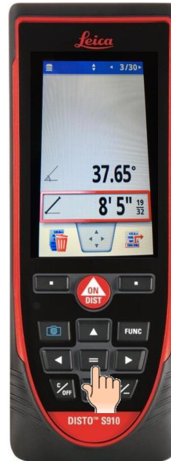
Once the red box is on the measurement, press the equals key.
