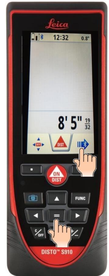
Now the measurement can be transferred by pressing touchscreen Bluetooth icon or pressing the equals key.
